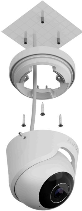
5. Place the camera enclosure in the holder, ensuring that the camera lens faces the protected area. Secure it in place by tightening the two screws in the holder using the bundled hexagon key ( $\varnothing$  2 mm).
