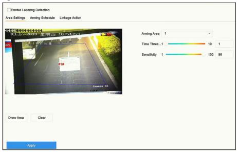
Figure 6-11 Loitering Detection
