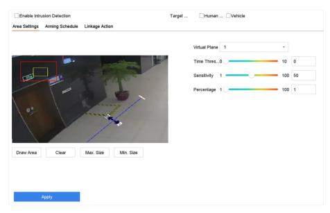
**Figure 6-7 Line Crossing Detection**
