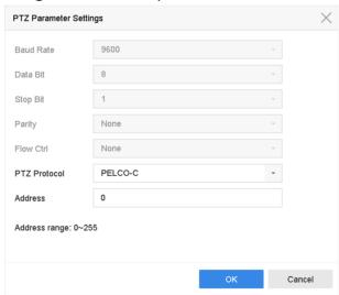
**Figure 3-5 PTZ Parameters Settings**
