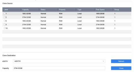
Figure 15-8 HDD Clone
