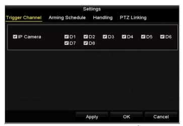
Figure 9-15 Set Trigger Cameras of POS
