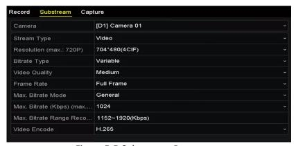
Figure 5-5 Sub-stream Parameters
