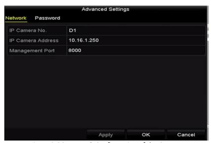
Figure 2-36 Network Configuration of the Camera
