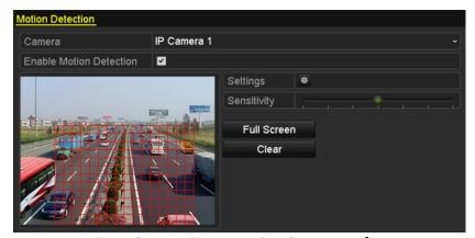
Figure 8-1 Motion Detection Setup Interface
