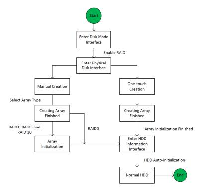
Figure 13-1 RAID Working Flow
