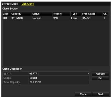
Figure 14-21 Disk Clone Configuration Interface
