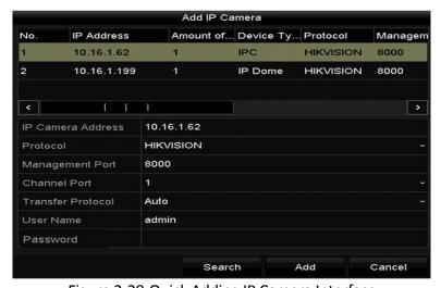
Figure 2-29 Quick Adding IP Camera Interface
