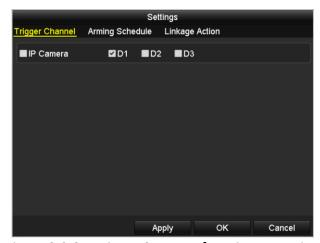
Figure 8-2 Set Trigger Camera of Motion Detection
