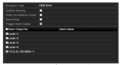
Figure 14-29 Configure HDD Error Alarm
