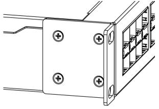
•Place the device in a rackmount enclosure and align with the holes so that the device fits conveniently.
